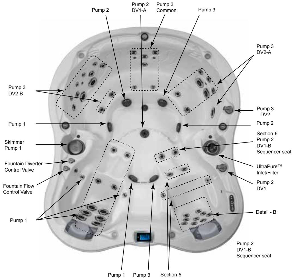
DV1 A =Diverter Valve 1 (A Position Clockwise)
